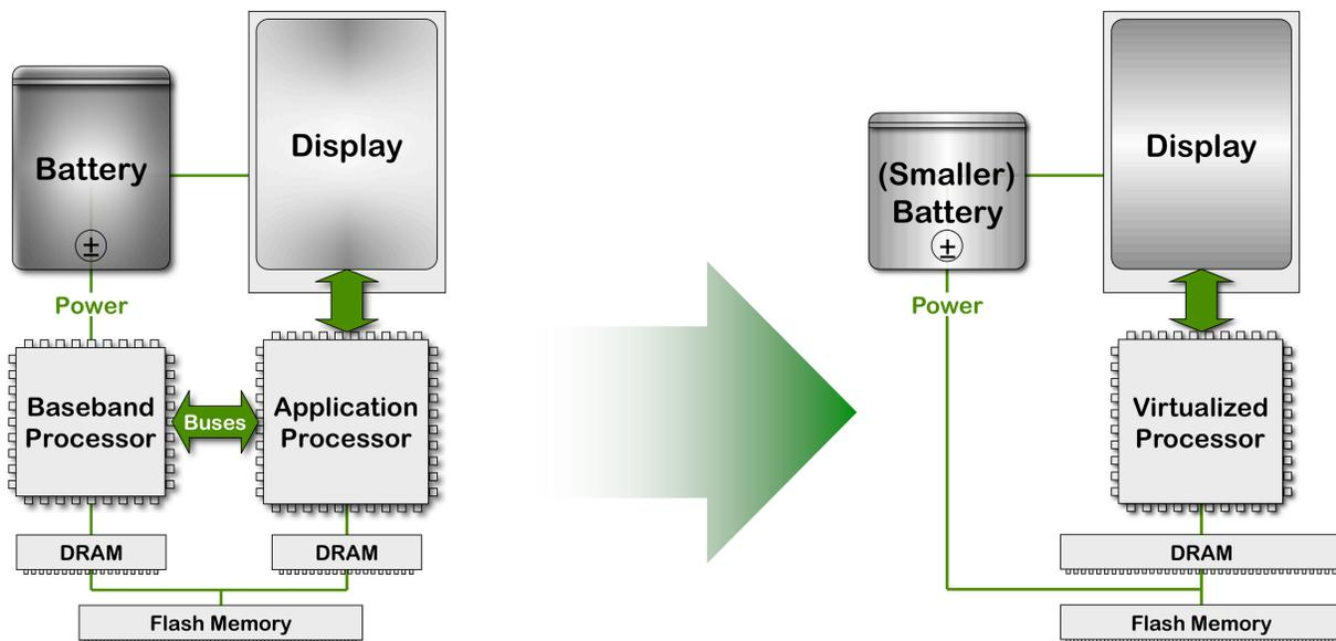
Figure 3. – Architecture Optimization with Mobile Virtualization
